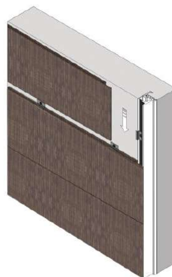
Installazione pannelli successivi Boiserie-H Installation of following panels Boiserie-H
