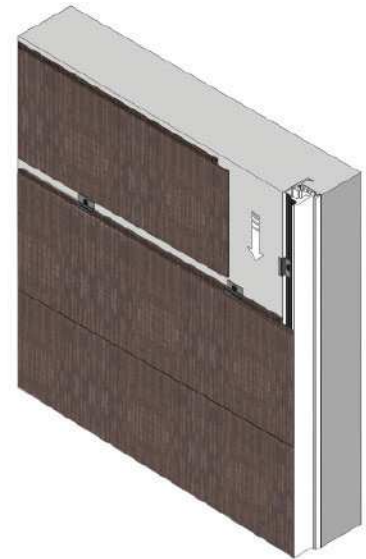
Installazione pannelli successivi Boiserie-H Installation of following panels Boiserie-H
